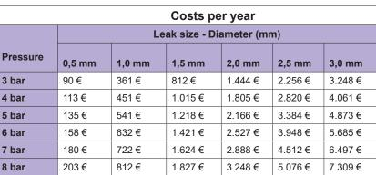
Table: Leakage costs within one year in case of operation 24 h/365 days, calculated with compressed air costs of 1.9 ct/Nm³.
